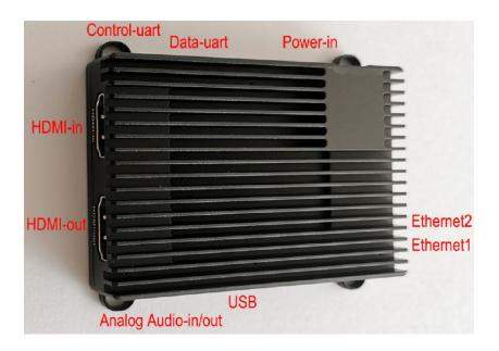
When S11 works as video encoder, it implements H.265/H.264 video encoding and audio codec, the stream will output via Ethernet after encoding. One channel uart data can also be packed with the stream and output to the Ethernet. The video encoding bitrates is controlled via control uart or web UI. S11 supports maximum 3840\*2160P@30 video encoding, and is downward compatibility for 3840P25/ 1080P60 / 1080P50 / ... video encoding.
