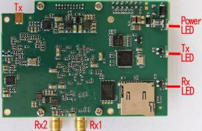
SEB1&DR2C module is a bidirectional transmission wireless link, it is composed of two independent unidirectional wireless channels, and the wireless links in both directions operate in different frequency bands. The wireless link itself does not have a handshake protocol, so when one direction of the wireless link is interrupted by interference, it does not affect the data transmission of the other direction of the wireless link. The Ethernet port supports TCP/UDP/IP protocols.
