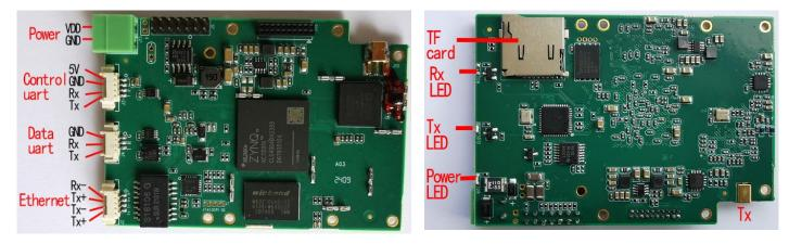
SEB1 Ethernet COFDM module accepts data from Ethernet port and transmits out. It can pair with SHD1&DR2C (or SHD4&DR2C, SEB1&DR2C) to implement one-way Ethernet/uart UDP data COFDM wireless transmission.
