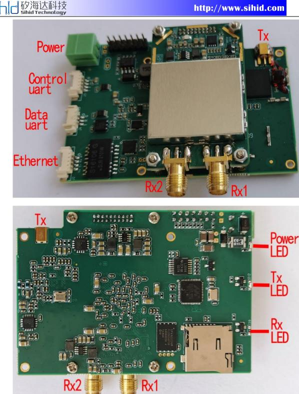
SEB1&DR2C can work as COFDM relay module or COFDM receiving module with Ethernet output, we have different firmware for it.
